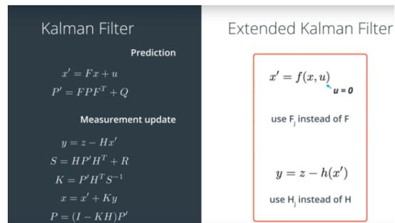
(b) Extended Kalman Filter v.s. Kalman Filter
