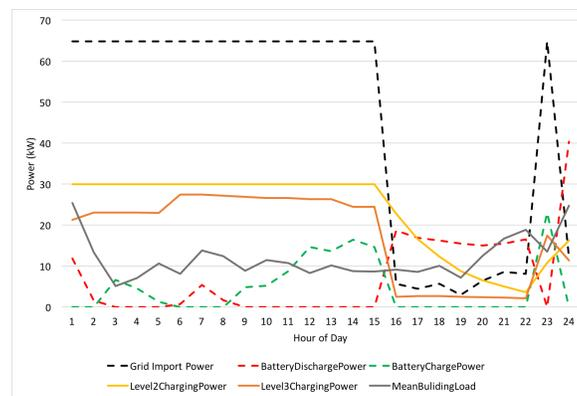
Figure 3: Optimal operation of a microgrid with EV charging using real data over 24 hours.
