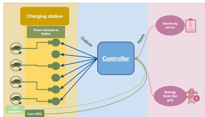
Figure 1: Description of the system's model
