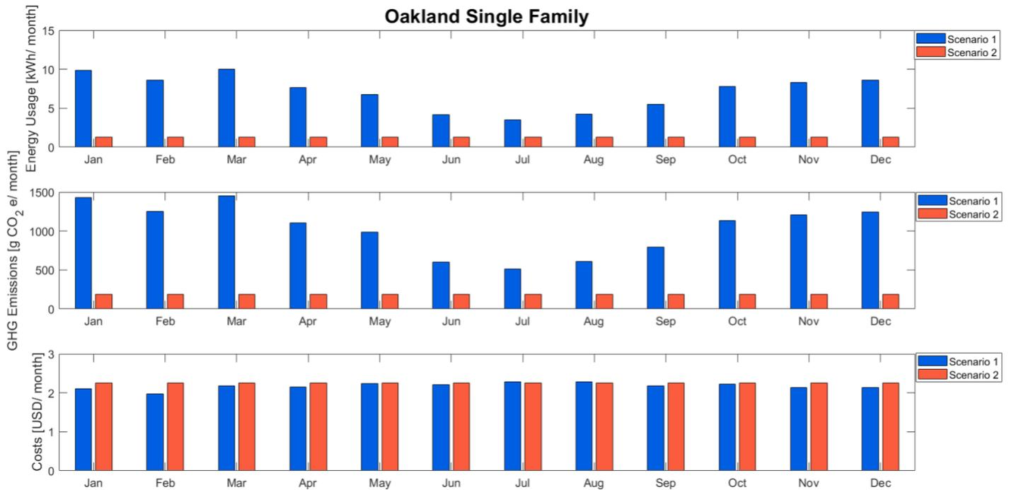
**Figure 6.** Energy intensity, GHG emissions, and cost comparison between the two modelled scenarios in Oakland.
