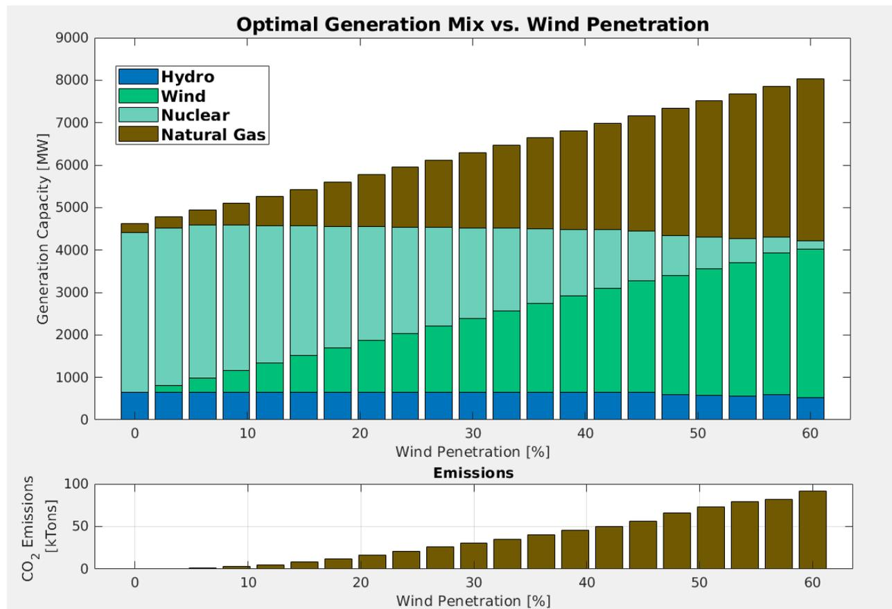
Figure 4: Optimal Generating Mix for Various Wind Penetrations, with Corresponding Emissions
