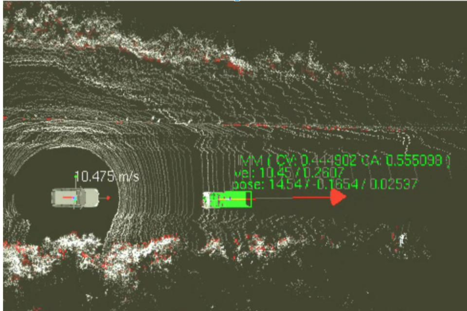
Figure 5: Tracked object (green) by Kalman filter
