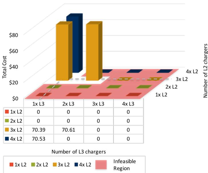
Figure 2: Optimal Size of Level 2 and Level 3 EV Chargers with Real Data. L2 and L3 reflect the number of Level 2 and Level 3 chargers, respectively. Total system cost is \$70 per day.
