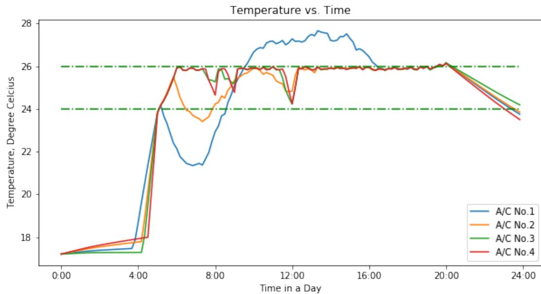
Figure 5: Interior Temperature under the Control of AC Units
