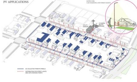
Figure 1: Schematic description of the microgrid
