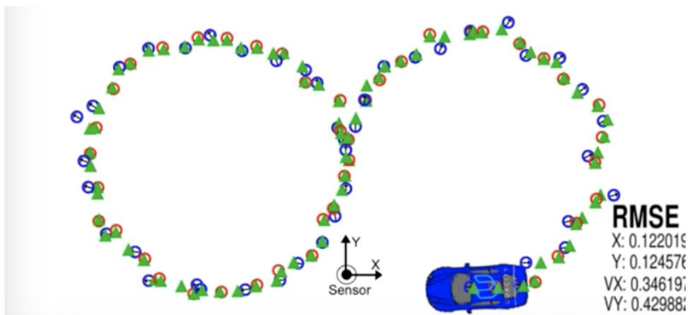
Figure 6: Estimation Results From LiDAR and Radar
