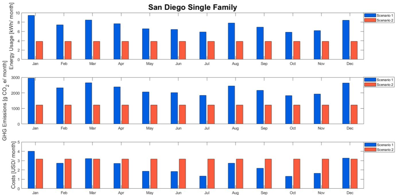
**Figure 7.** Energy intensity, GHG emissions, and cost comparison between the two modelled scenarios in San Diego.
