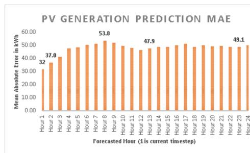
Figure 11: Forecast Error for Each Hour in the Prediction Horizon. MAE is 12.3% of Test Maximum Hourly Energy Generation
