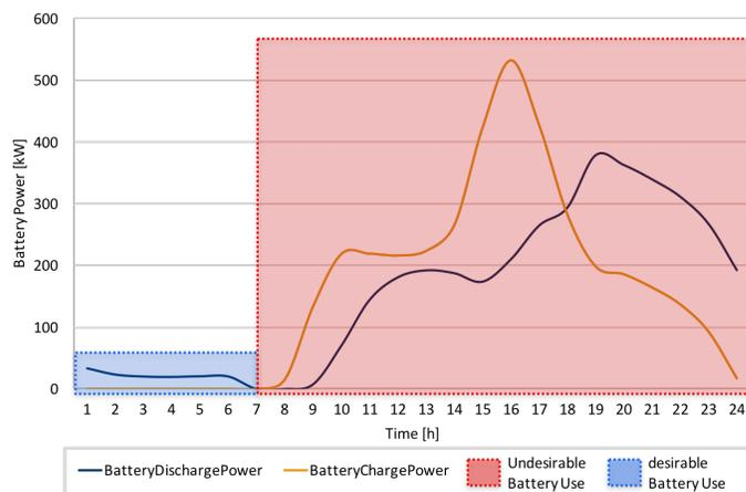
Figure 5: A Example Corner Case of Simultaneous Charging and Discharging of Battery. Blue regions indicate desired behavior while red shaded regions indicate undesirable battery behavior, i.e., simultaneous charging and discharging.
