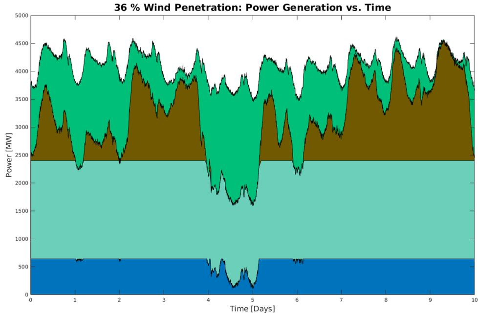
Figure 2: Effect of moderate penetration of Wind generation on the overall generation for 10 day period
