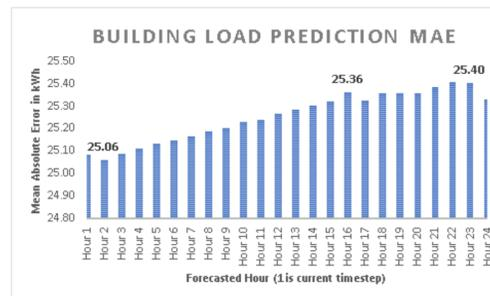
Figure 12: Forecast Error for Each Hour in the Prediction Horizon. MAE is 24.6% of Test Maximum Hourly Energy Demand
