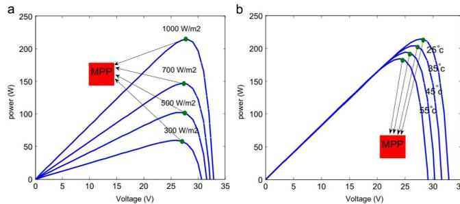
Figure 4: Power–voltage curve of a PV module for different conditions of solar irradiance and cell temperature [12].
