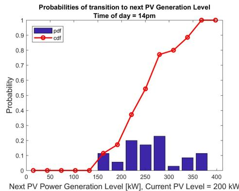
Figure 6: Transition probabilities for a specific solar power generation level and specific time of day
