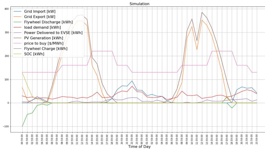
Figure 20: MCP operations simulation with only 3-hour time horizon
