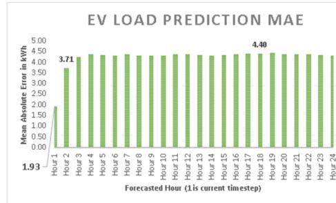
Figure 10: Forecast Error for Each Hour in the Prediction Horizon. MAE is 11.7% of Test Maximum Hourly Energy Demand
