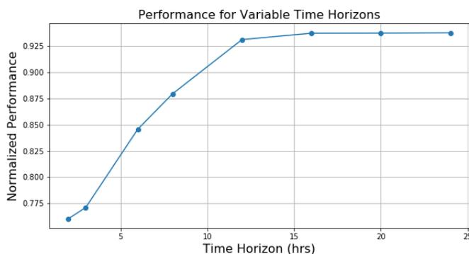
Figure 15: Normalized performance of MCP when varying time horizons used.
