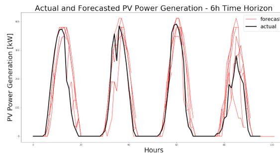
Figure 7: Forecasted solar power generation values using a 6h-time-window (red) and actual solar power generation values (black)
