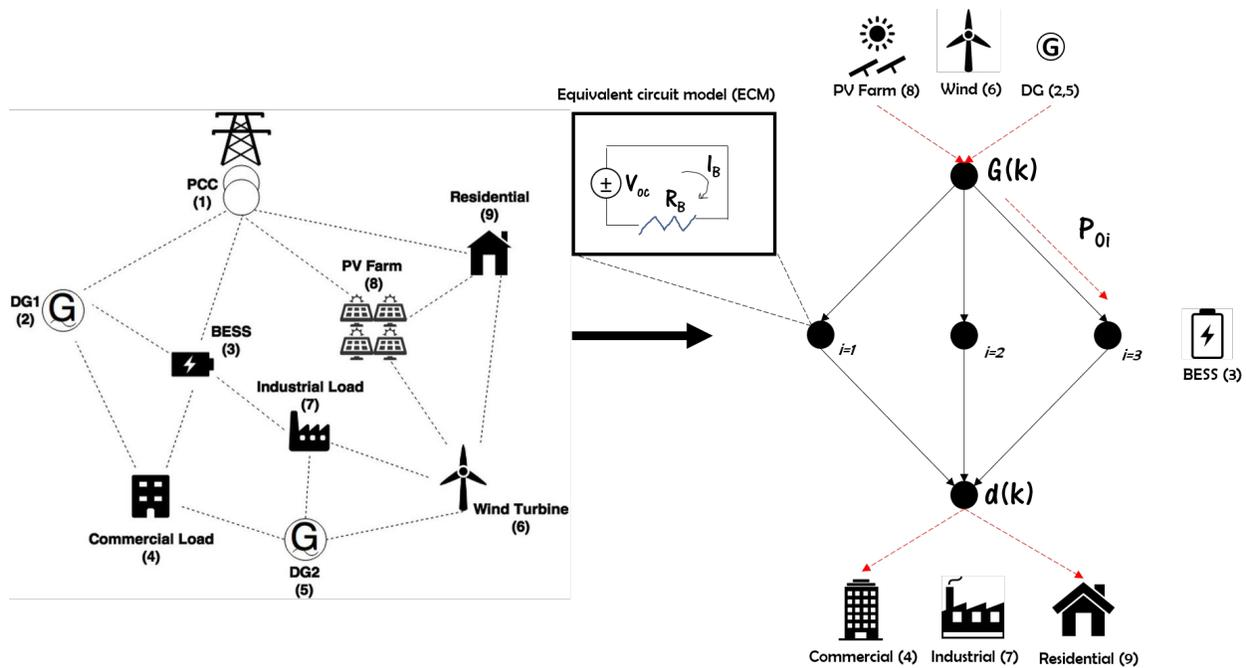
**Figure 2.** Grid transformation of a typical microgrid network into a max flow problem. The inherent assumption is that we use prior knowledge on the evolution of  $G(k)$  and  $d(k)$  as supply and demand. The remaining surplus or shortage will be taken from the batteries at each node  $i$ . Figure adapted from [8].
