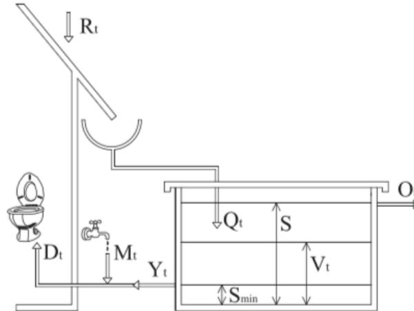
**Figure 2.** Rainwater harvesting mathematical model, to be used at a daily timestep. Adapted from: Palla, A; Gnecco, I; and Lanza, L.G. 2011. Non-dimensional design parameters and performance assessment of rainwater harvesting systems. *Journal of Hydrology*. 401, 65-76. Accessed on 2/6/2018 at 11:00 P.M.
