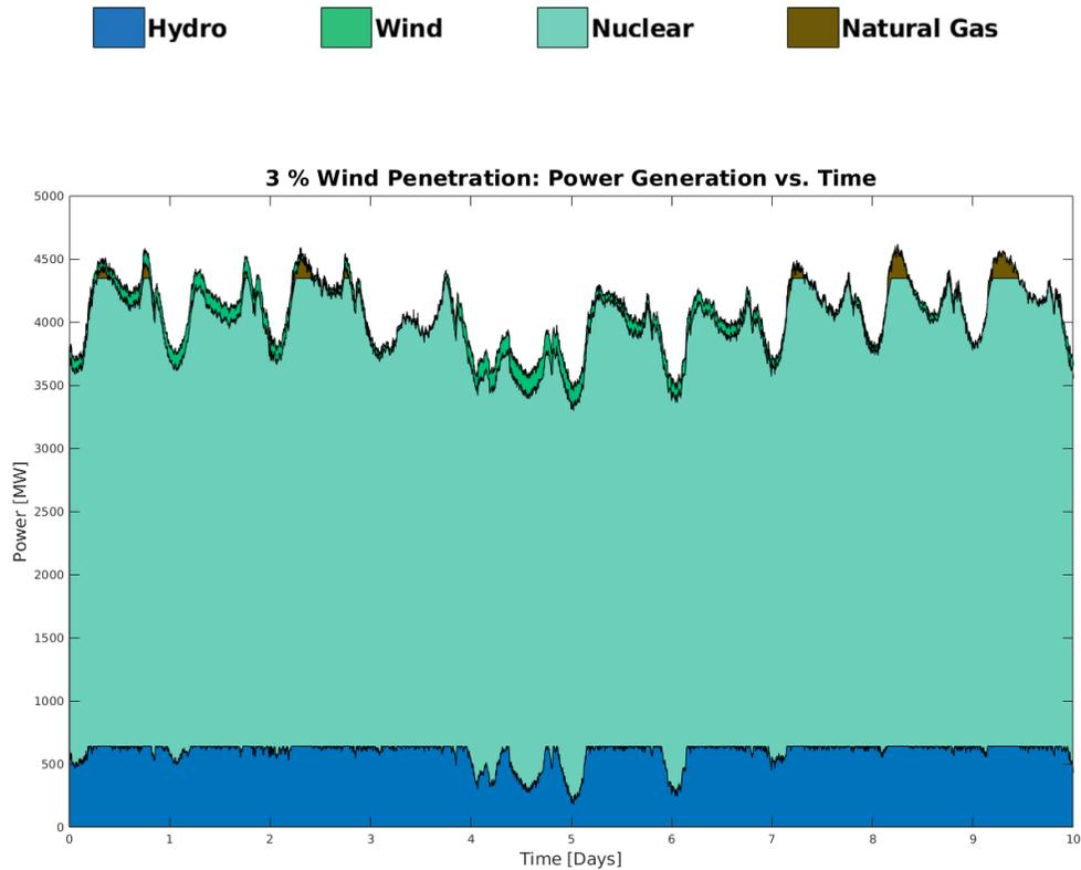
Figure 1: Effect of low penetration of Wind generation on the overall generation for 10 day period
