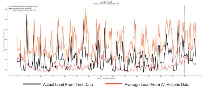
Figure 9: Forecast model output for building load demand compared to actual test data and average from all historic data.
