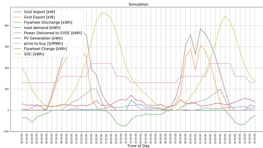
Figure 21: MCP operations simulation with full 12-hour time horizon
